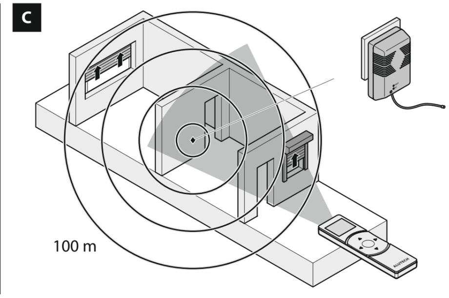
**EN** The AR-S signal repeater serves to increase the signal range of an ALUTECH remote control when communicating with a radio receiver (of an electric drive, control unit, etc.) in areas with weak radio penetration.
